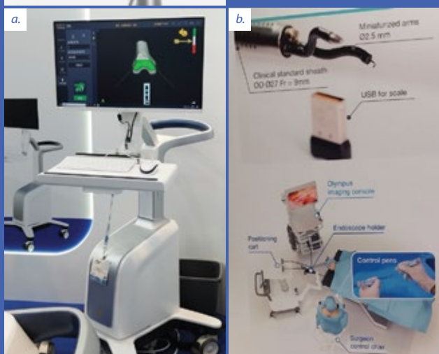
Figure 2. Two typical "slave-master" robotic systems a) for orthopaedic surgery and b) for endoscopic procedures. Both systems are operated by the surgeon with fine pen or grip style remote control devices.
