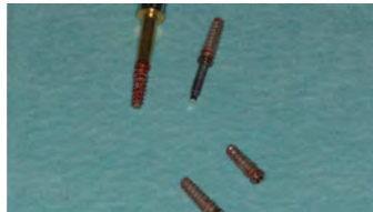
Extracted failed implants
