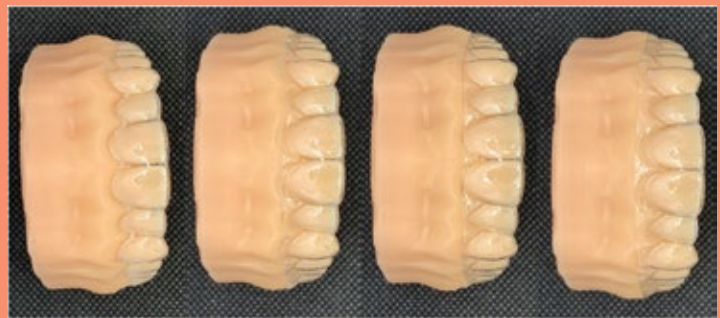
Fig. 2. Different designs of trimming line of orthodontic aligners; from Left to Right: Scalloped, Scalloped Extended (2 mm), Straight, and Straight Extended (2 mm).
