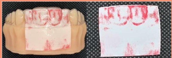
Fig. 3. Pressurized Fuji Prescale pressure sensitive film used for investigating the stress distribution map generated by clear aligner on the surface of a 0.2 mm facially malaligned upper right central incisor (Tooth 11) of a 3D-printed model.
